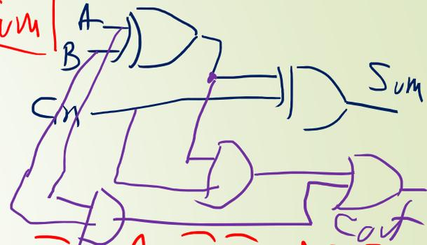
$$S = \bar{A}\bar{B}C + \bar{A}B\bar{C} + A\bar{B}\bar{C} + ABC$$
